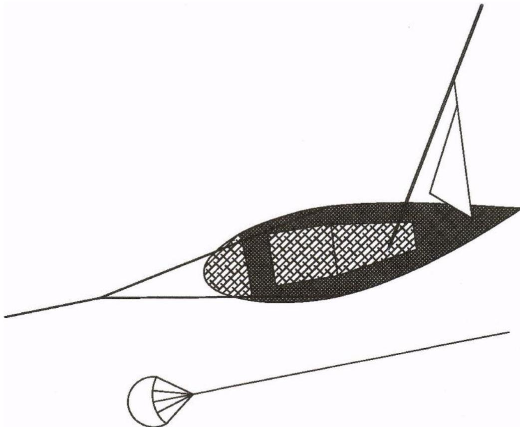
Sketch shows small parachute anchor used as drogue. Bridle lines led to port and starboard main winches can provide emergency steering. *Product obtained from a specialist supplier is recommended.*
